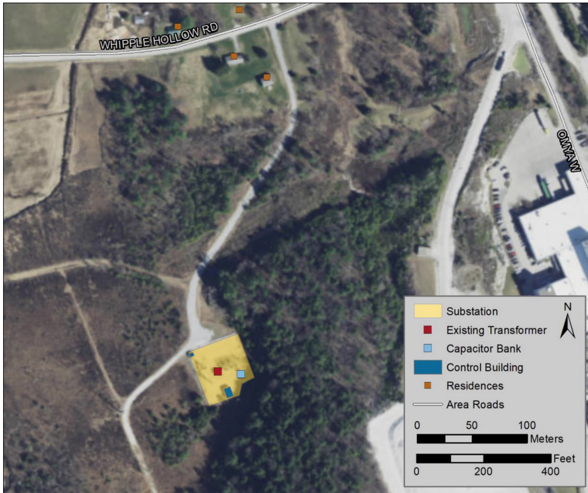
FIGURE 2: MAP OF EXISTING SUBSTATION LAYOUT
