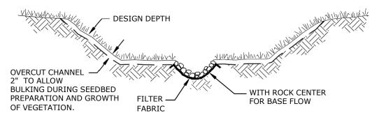
TYPICAL TRAPEZOIDAL CHANNEL CROSS-SECTION
