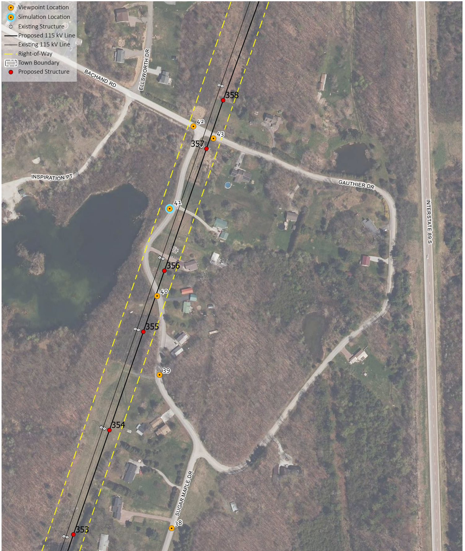
VELCO Franklin County Line Upgrade - MAP 13: Gauthier Drive Corridor Crossing - Swanton, VT
